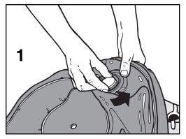
Locate base filler area and remove the filler cap.
